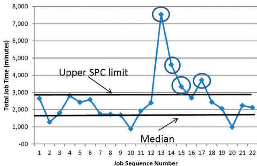
This chart shows the total job time for 22 jobs and the expected median and upper limits. Using a technique known as statistical process control, in this example, four jobs that fall outside the expected limits have been identified. These are candidates for further investigation and remedial action.
