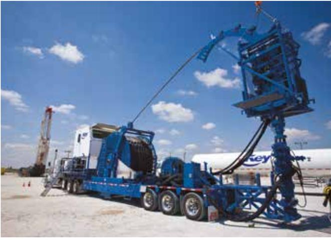
**Figure 1.** A Key Energy Services coiled tubing unit. The spooled continuous pipe can reach lengths of up to 48 000 ft for the smaller diameters (1.25 in.) and is used to convey tools, log, stimulate, clean-out and perform other Intervention functions in oil and gas wells.
