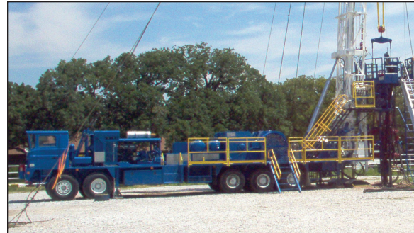
Class III scoping mast service rig; Derrick Ht up to 112'
